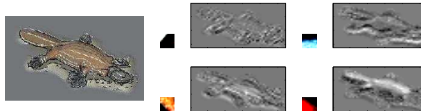
Figure 4. Left: An example platypus image from the Caltech 101 dataset. Right: Features computed for the platypus image using four sample image patch bases (trained on color images, and shown in the small colored squares) by computing features at different locations in the image. In the large figures on the right, white pixels represents highly positive feature values for the corresponding basis, and black pixels represents highly negative feature values. These activations capture higher-level structure of the input image. (Bases have been magnified for clarity; best viewed in color.)
