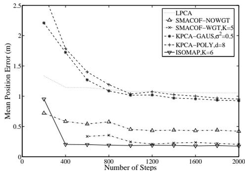
Figure 4. Transition of Mean Position Errors in Visibility-Only Mapping (LPCA,SMACOF,KPCA,ISOMAP)
