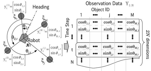
Figure 3. Bearing-Only Measurements
