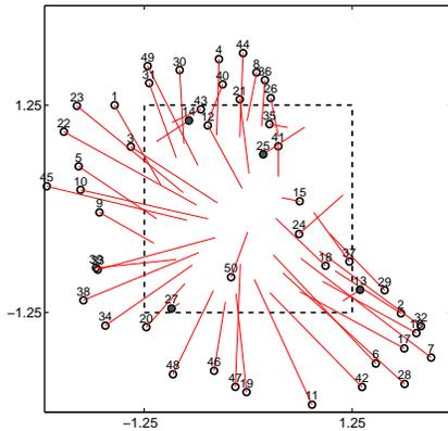
Figure 6. A Map Built by LPCA in Visibility-Only Mapping After 2000 steps (MPE:1.023m, MOE:15.95%)
