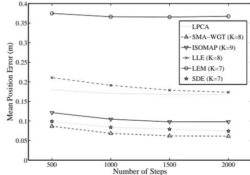
Figure 8. Transition of Mean Position Errors in Bearing-only Mapping (LPCA, SMACOF, ISOMAP, LLE, LEM, SDE)
