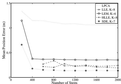
Figure 5. Transition of Mean Position Errors in Visibility-Only Mapping (LPCA,LLE,LEM,HLL,SDE)
