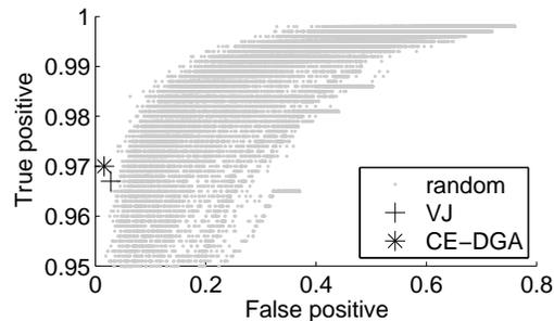
Figure 3. The ROC domain. The performances of randomly drawn parameters, Viola-Jones parameters (VJ), and parameters optimized by the CE-DGA method, respectively, shown in the True Positive Rate  $\times$  False Positive Rate coordinate system.
