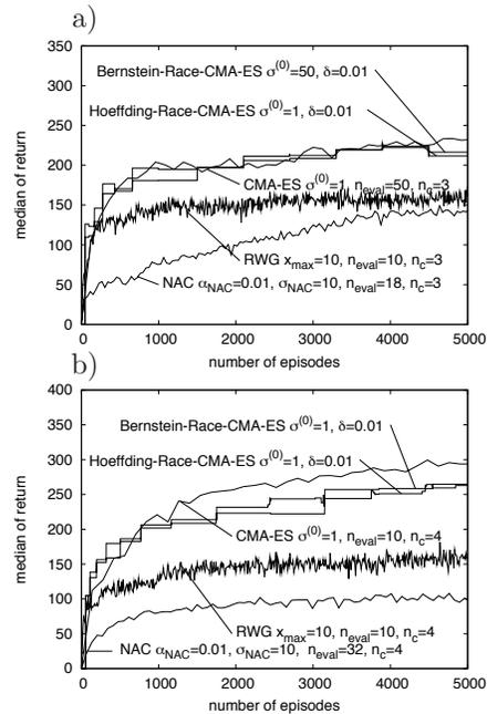
Figure 3. Median of performance over 20 trials for RWG, NAC, CMA-ES, Bernstein-Race-CMA-ES, and Hoeffding-Race-CMA-ES for swimmers with a) 3 and b) 4 segments. The respective best parameter configuration is plotted.
