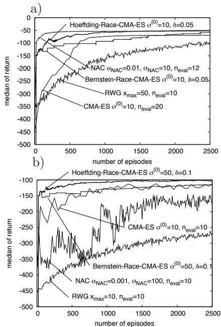
Figure 2. Median of performance over 500 trials for RWG, NAC, CMA-ES, Bernstein-Race-CMA-ES, and Hoeffding-Race-CMA-ES in the a) fully observable and b) partially observable mountain car task. The respective best parameter configuration is plotted.
