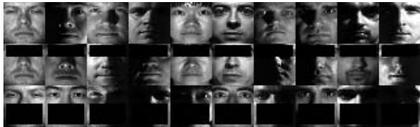
Figure 1. Selected sample images without and with artificial outliers in the YaleB set. Top row: clean images; Middle row: outliers by forehead and eyes occlusion; Bottom row: outliers by nose and mouth occlusion.
