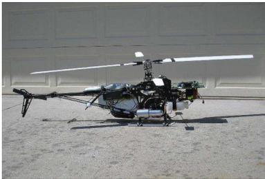
Figure 7. Tempest autonomous helicopter.
